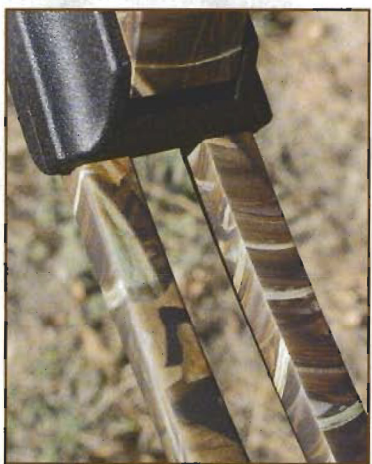
A strong dose of high-tech can be found in the Menace's machined riser, molded limb cups and split limbs.
