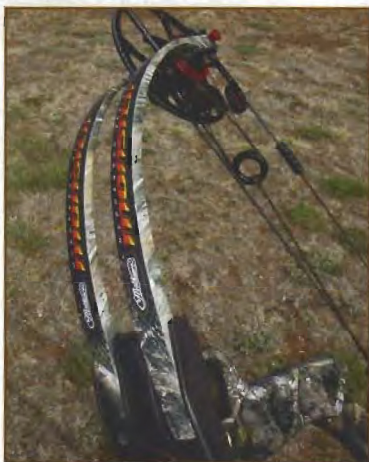
Dramatically pre-loaded 14-inch limbs on the Monster are locked into self-aligning limb pockets, and their past-parallel configuration helps dampen shot vibration and noise.
