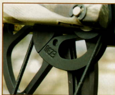
Interchangeable modules make for convenient and easy draw-length adjustments with the Parker BlackHawk EZ-Draw.
