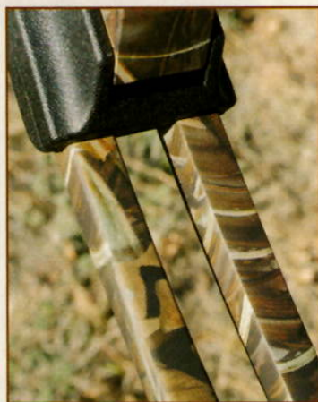
A strong dose of high-tech can be found in the Menace's machined riser, molded limb cups and split limbs.
