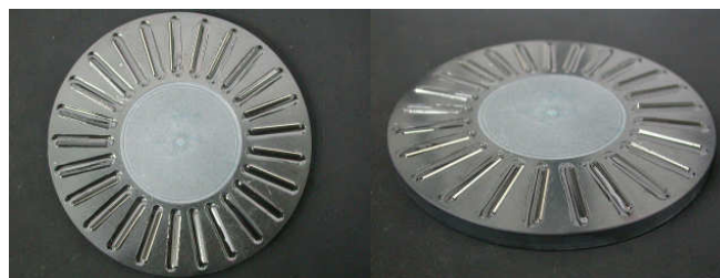
Figure 8. The UDD with the design of sliding blades. Multiple design features can be accommodated with number of blades and tilt angles.
