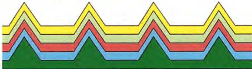
Figure 37 The resharpening of ADD cutting pyramids after each use to duplicate the same profile (see online version for colours)
