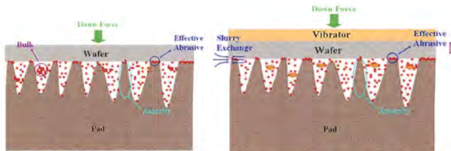
Fig. 10: The illustration of ultrasonic effects on the dispersion of slurry in the asperities of pad surface.
