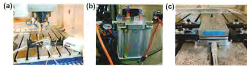
Figure 3. (a) Photo of experimental setup; (b) details of MQL equipment [1-export of pure water mist, 2-filler, 3-knob for lubricant flow rate adjustment, 4-window for viewing droplets, 5-manometer (0–150 psi or 0–10.2 kgf/cm 2 ), 6-water meter, 7-air inlet]; and (c) dynamometer setup.
