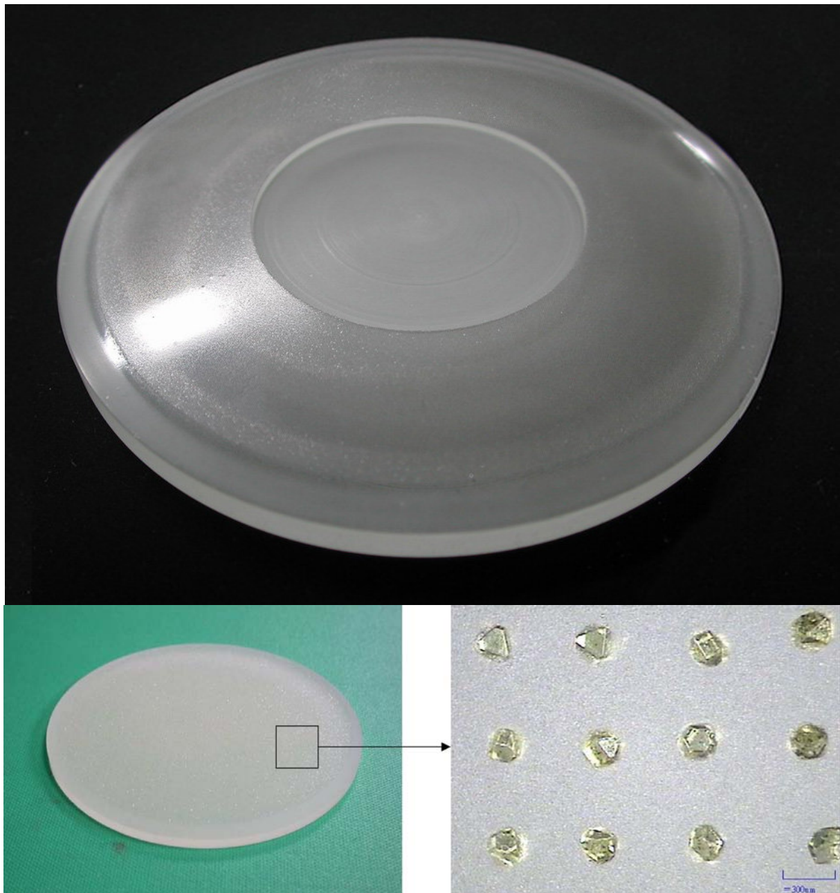
Fig. 2: Transparent ODD can allow defects (e.g. missing diamond) be spotted with naked eyes.
