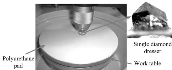
FIGURE 5 Schematic drawing of dressing test.
