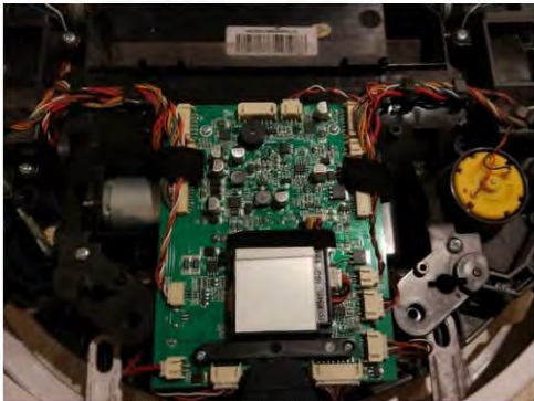
Motor Control DCDC BMS
