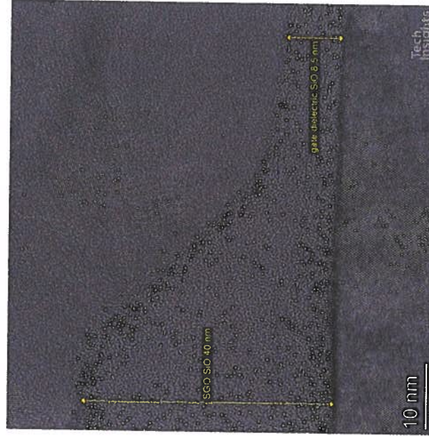
HS/LS FET Gate Dielectric – TEM Cross-Section
