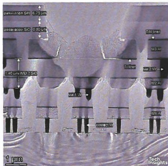
Passivation and Metal 3 – TEM Cross-Section
