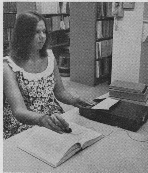
Fig. 1. Portable model of the reading aid. This model, designed for personal use by a blind person, incorporates the features of the previously described models of the reading aid plus battery operation, adjustable magnification, and reduced size.
