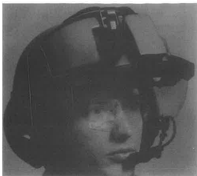
Figure 12. Two optical see-through HMDs, made by Hughes Electronics.
