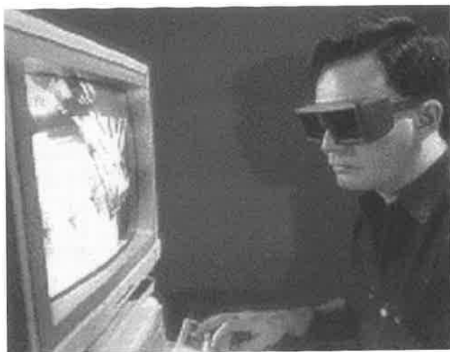
Figure 16. External view of the ARGOS system, an example of monitor-based AR. (Courtesy David Drascic and Paul Milgram, U. Toronto.)
