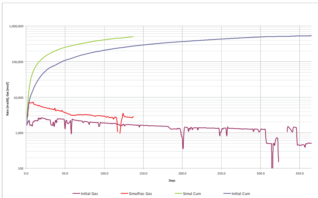
Figure 20 – Project 2 average gas rate and cumulative production for the single well completions and the offsetting simultaneously fractured wells.
