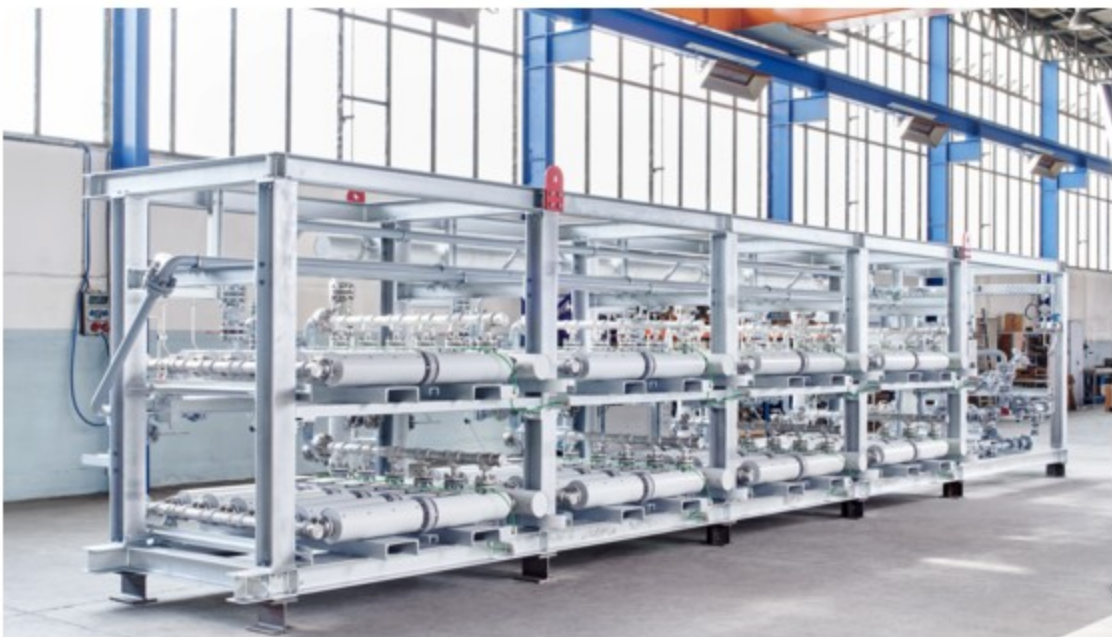
HISELECT® powered by Evonik membrane skid built for a petrochemical complex in Texas, United States of America
