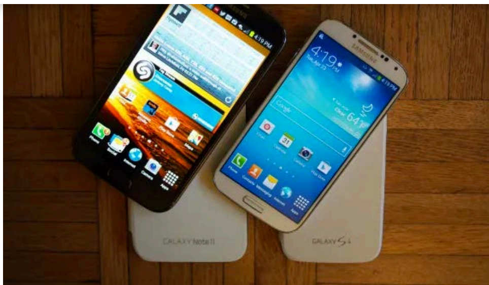
5.5-inch 720p HD display of the Galaxy Note II on left compared with 5-inch 1080p display of the Galaxy S4 on the right.
