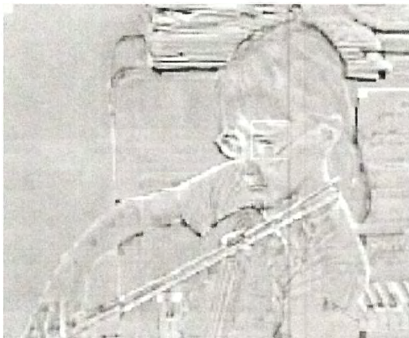
Figure 6.8 Residual after subtracting intra prediction
