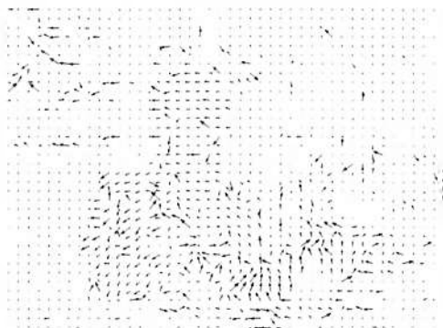
Figure 3.22 Motion vector map : 4 \times 4 blocks, 1/4-pixel vectors
