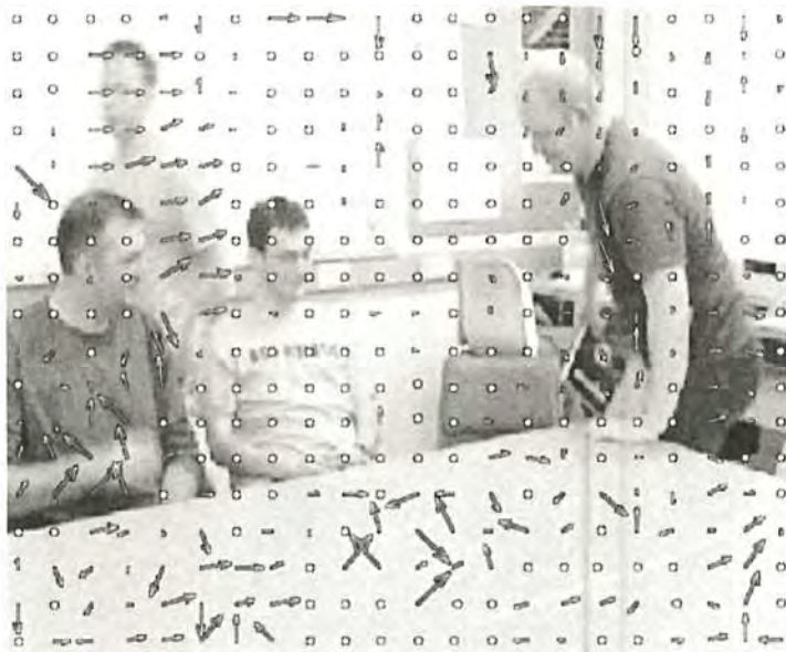
Figure 3.56 16 \times 16 motion vectors superimposed on frame
