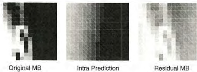
Figure 4.8 Original macroblock, intra prediction and residual
