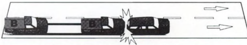
Light truck with rear wheel anti-lock braking system (some stability, front wheels lock, still unsteerable)
