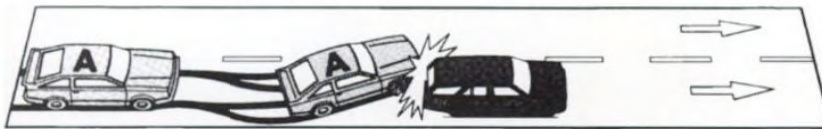
Car without anti-lock braking system (all wheels lock, skidding, unsteerable)
