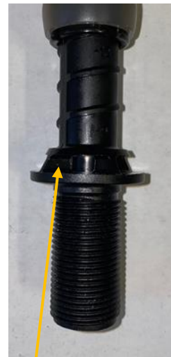
tank water outlet
