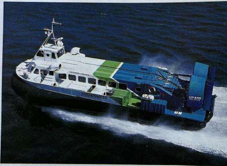
Figure 4-5 A hovercraft floats on a cushion of air above the water. Air provides less resistance to motion than water does.
