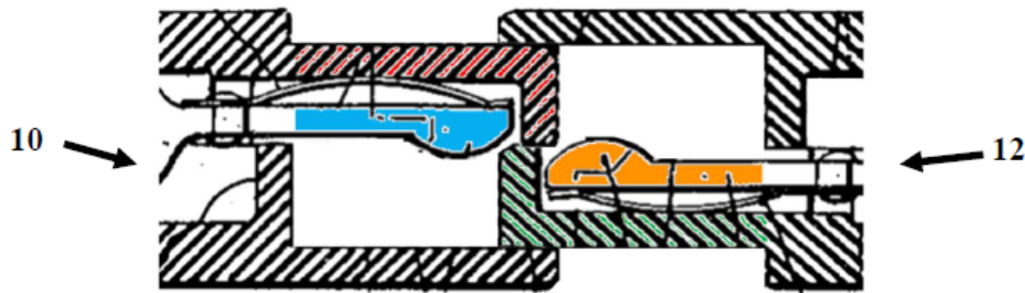
Diagram created based on Ex. 1004, Fig. 2, (modified to show connector 10 and connector 12 partially disconnected)
