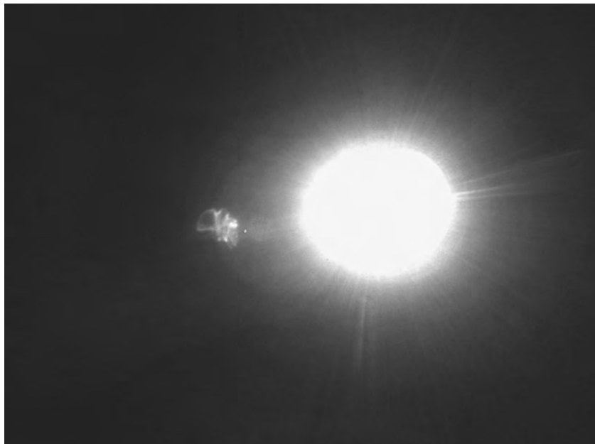
Figure 24.3 Commercial Digital Camera Exhibiting Scatter Artifacts in Pres- ence of Very Bright Flashlight Object. Note the Bright Halo and Scatter Spot
