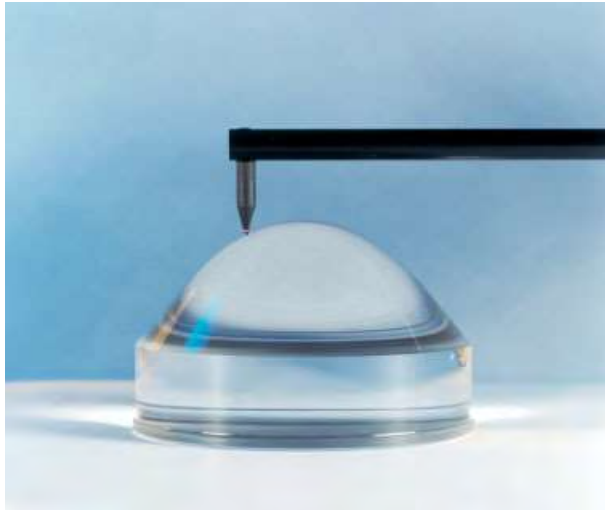
Figure 4.9 Contact profiling (photo courtesy of Taylor Hobson Ltd. [27]).
