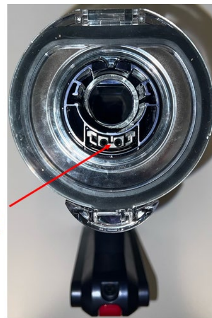
Cyclone unit electrical connector
