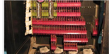
CPU, core memory, and external bus interface of a DEC PDP-8, all made of medium-scale integrated circuits
