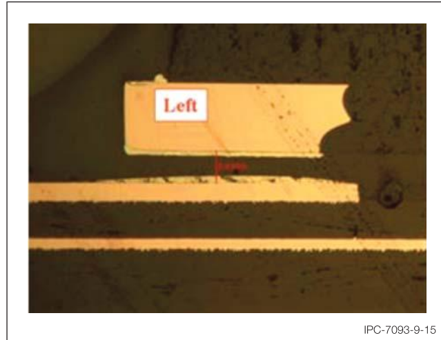
Figure 9-15 Tilted BTC causing high joint height open on the left.
