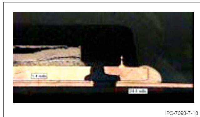
Figure 7-13 Post Assembly Contact and DAP Solder Joint Profile
