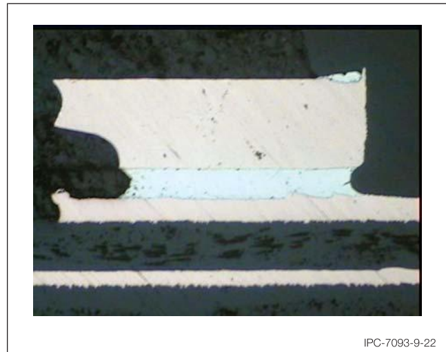
Figure 9–22 No Side fillet on bottom termination component.
