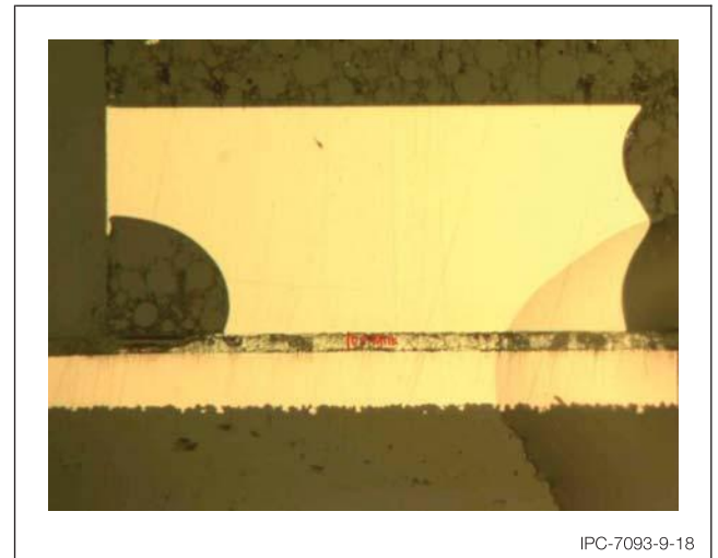
Figure 9-18 Half etched option on BTS component.
