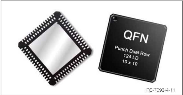
Figure 4-11 Fine-Pitch Two Row QFN (No lead) Packaging
