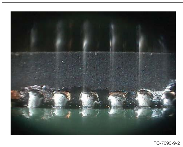
Figure 9-2 Optical image of acceptable QFN edge terminations. Solder fillets should be visible to a minimum of 75% of the width of the termination.
