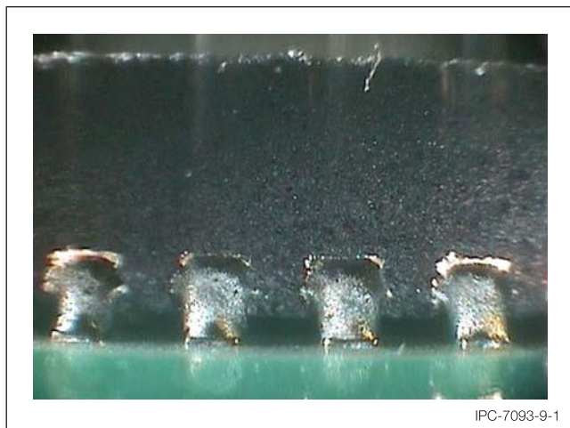
Figure 9-1 Optical image of acceptable QFN edge terminations. Solder fillets should exist if the design incorporates pads that extend beyond the package width.
