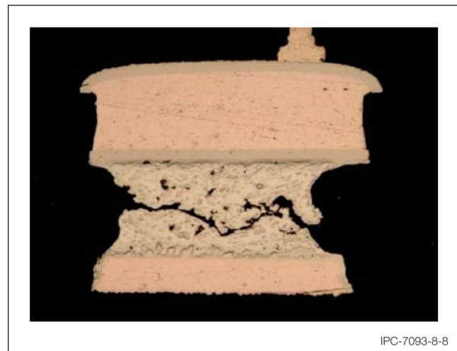
Figure 8-8 Solder Crack Due to Cte Mismatch after 1000 Cycles
