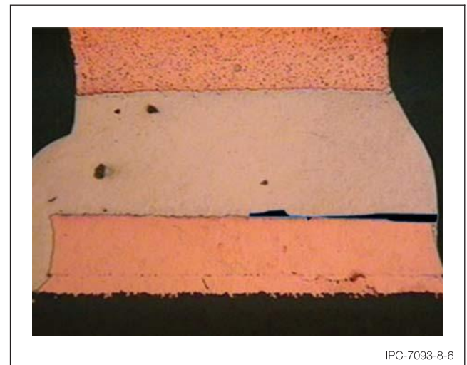
Figure 8-6 The Crack Formation is the Result of the CTE Mismatch
