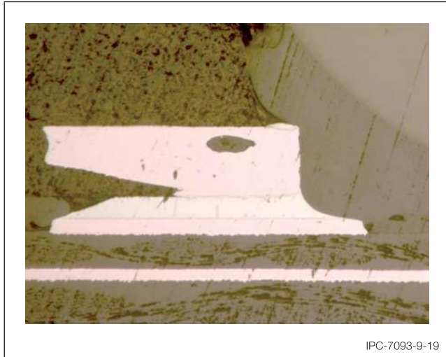
Figure 9–19 Small fillet due to nonwetting of the side copper.
