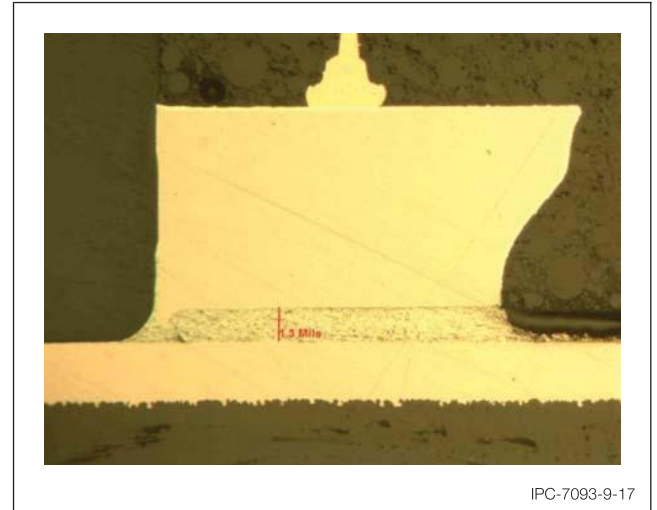
Figure 9-17 Full lead option on BTS component.
