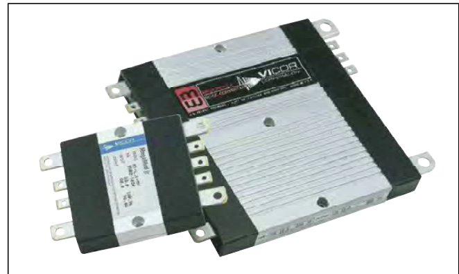
Figure 24-4 — MegaMods housing assembly
