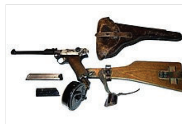
Artillery Luger P08 pistol with snail-drum magazine and removable stock.
