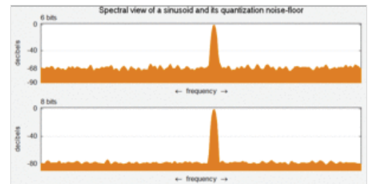
Comparison of quantizing a sinusoid to 64 levels (6 bits) and 256 levels (8 bits). The additive noise created by 6-bit quantization is 12 dB greater than the noise created by 8-bit quantization. When the spectral distribution is flat, as in this example, the 12 dB difference manifests as a measurable difference in the noise floors.
