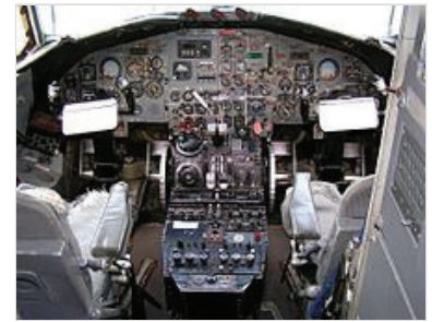
The BAC-111 cockpit includes a stick shaker/pusher following its 1963 crash
