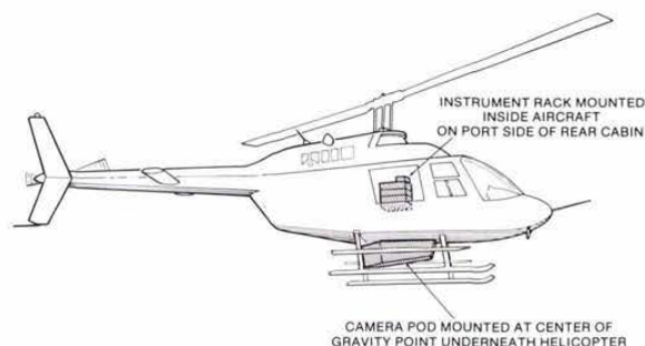
FIG. 1. Illustration of camera pod and instrument rack installed on helicopter.
