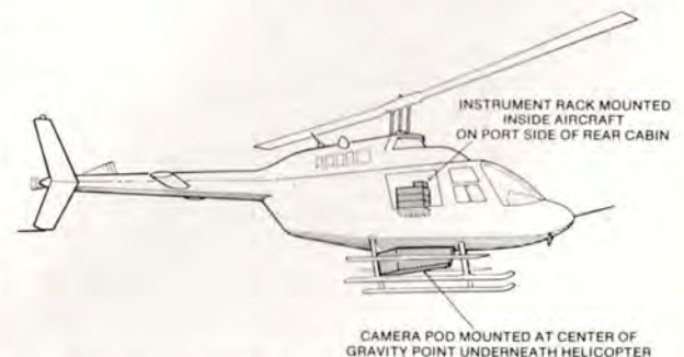
FIG. 1. Illustration of camera pod and instrument rack installed on helicopter.
