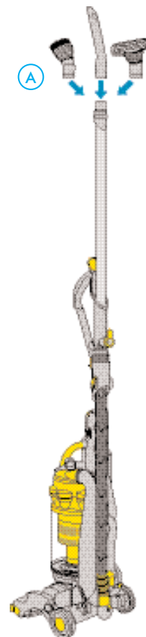
A Tools can be fitted directly to the end of the wand and hose for cleaning hard to reach places.
