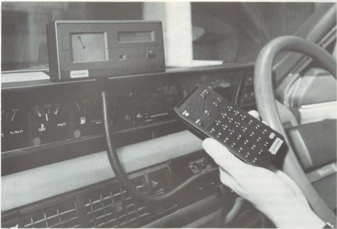
Fig. 43.3 The Autoguide screen (courtesy Department of Transport).
