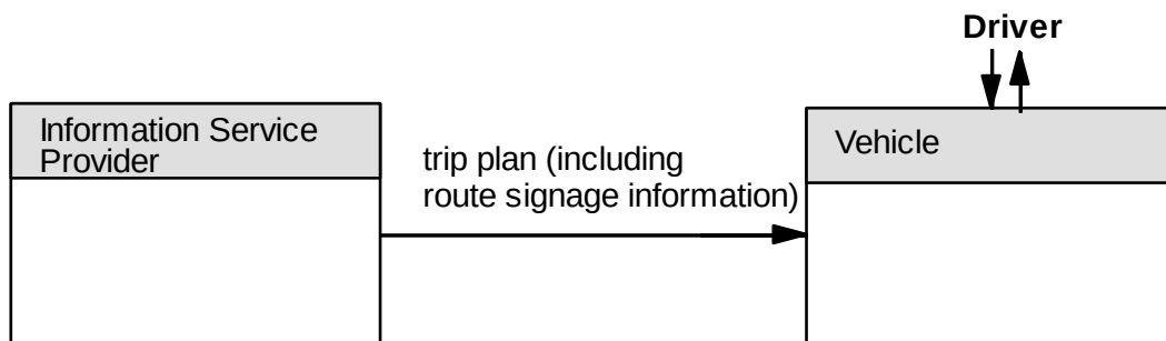
Figure 7 - Alternative Physical Architecture for In-Vehicle Signage
