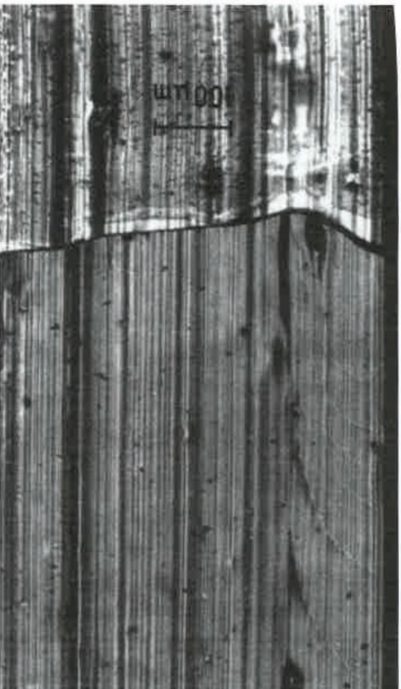
Figure 11. Spalled spot of SiC coating from the Pitch-55 ribbon.
