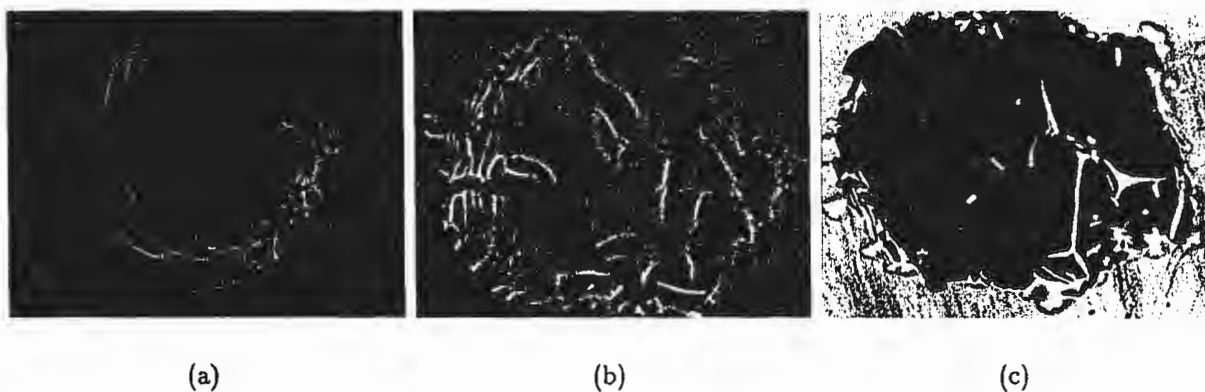
Figure 4.11: Damage patterns observed on a 1.2 \mu\text{m} thick aluminum film with a 6 \mu\text{m} thick waterglass confining layer and laser fluence of: (a) 0.084 J/mm 2 ; (b) 0.112 J/mm 2 ; (c) 0.140 J/mm 2 .
