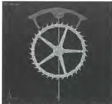
Fig. 1: Model of Graham Escapement in RecurDyn®.
