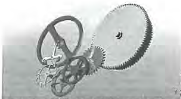
Fig. 7: The model of Swiss Lever Escapement connected to the gear train and the barrel. The escapement is on the left side while the barrel is on the right.
