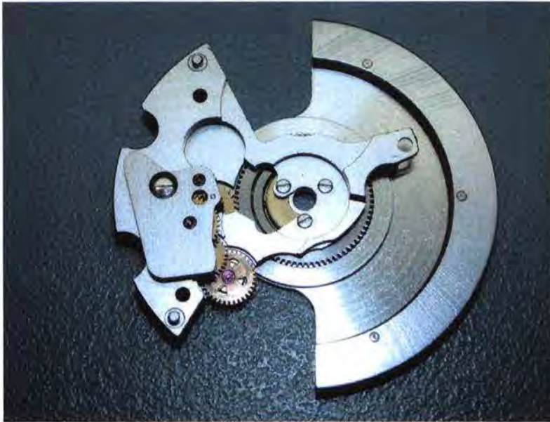
Figure 42: “Double Wheels and Pinions System” of ETA mechanical watches. [41]
