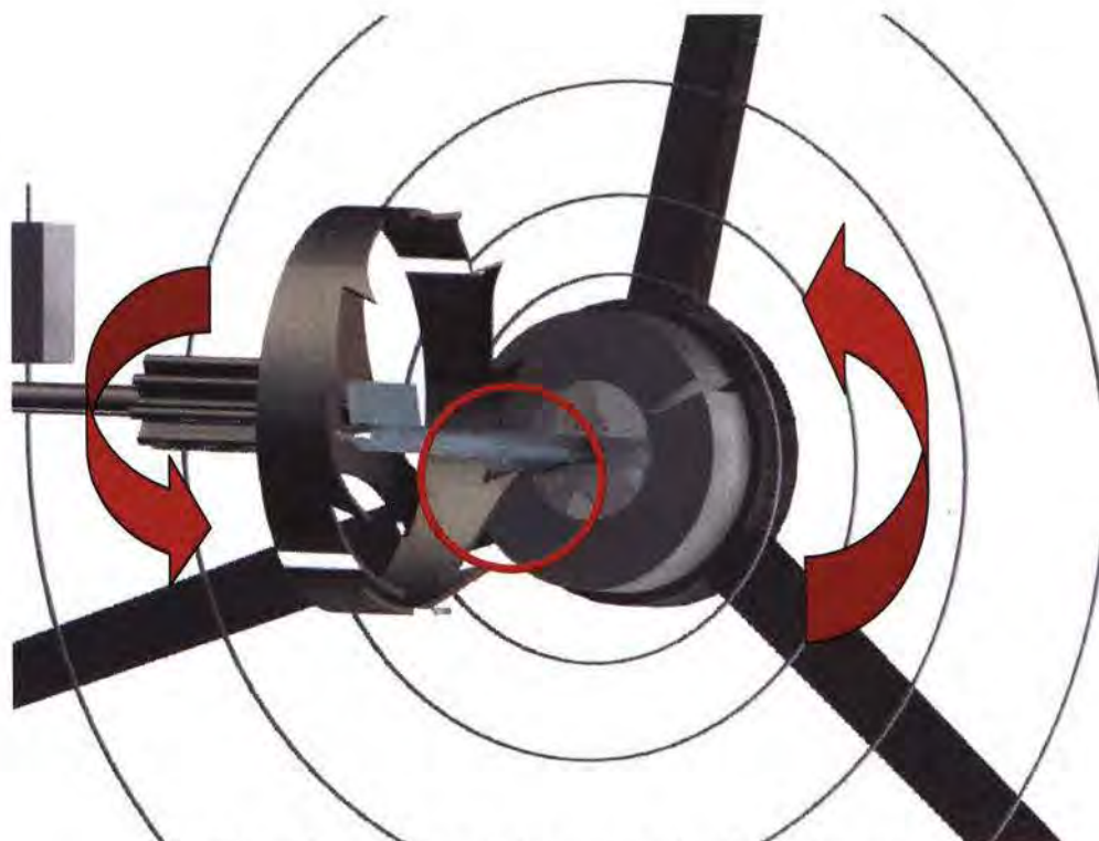
Figure 35: Locking of the escape wheel's back tooth.
