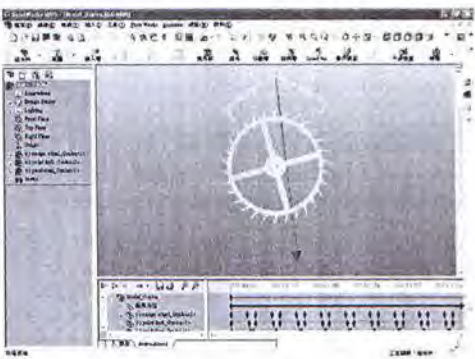
Fig. 16: The animation setting interface in SolidWorks® with the Graham Escapement
