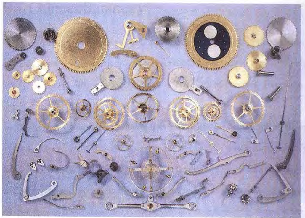
Figure 55: Moon phase mechanism components with 135 teeth moon phase disc. [27]
