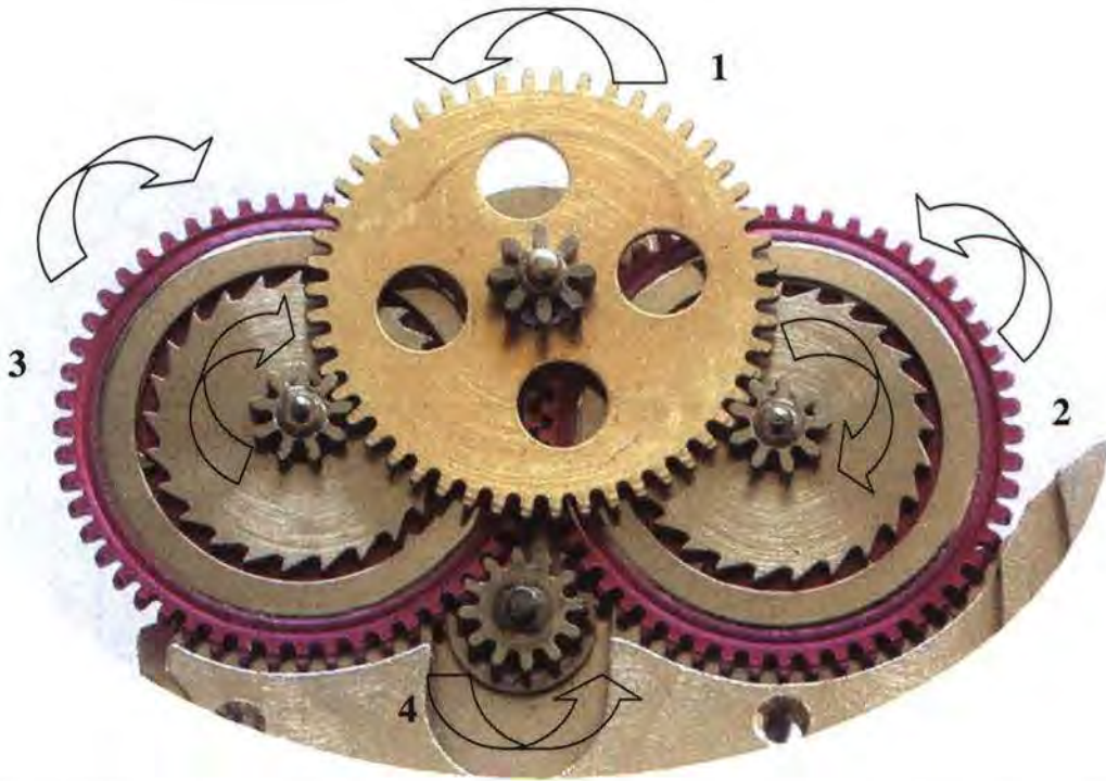
Figure 39: Automatic winding system of Rolex – rotor rotates anti-clockwisely. [39]
