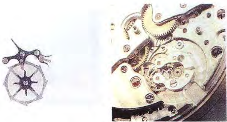
Figure 17: Daniels Co-Axial Double-Wheel Escapement in a mechanical watch with 2mm thickness. [27]
