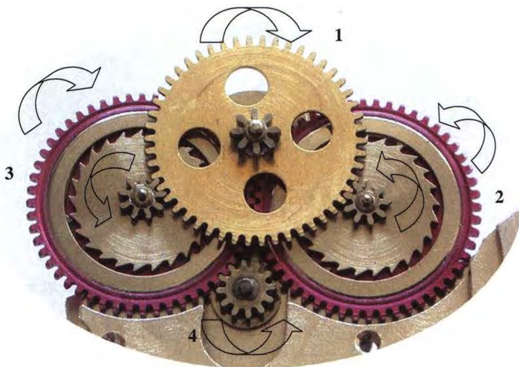
Figure 38: Automatic winding system of Rolex – rotor rotates clockwise. [39]
