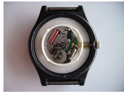
Basic quartz wristwatch movement Bottom right: quartz crystal oscillator , left: button cell watch battery, top right oscillator counter, digital frequency divider and driver for the stepping motor (under black epoxy), top left the coil of the stepper motor that powers the watch hands.
