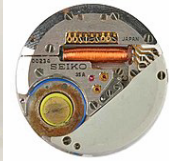
First quartz wristwatch movement, Caliber 35A, Seiko, Japan, 1969
