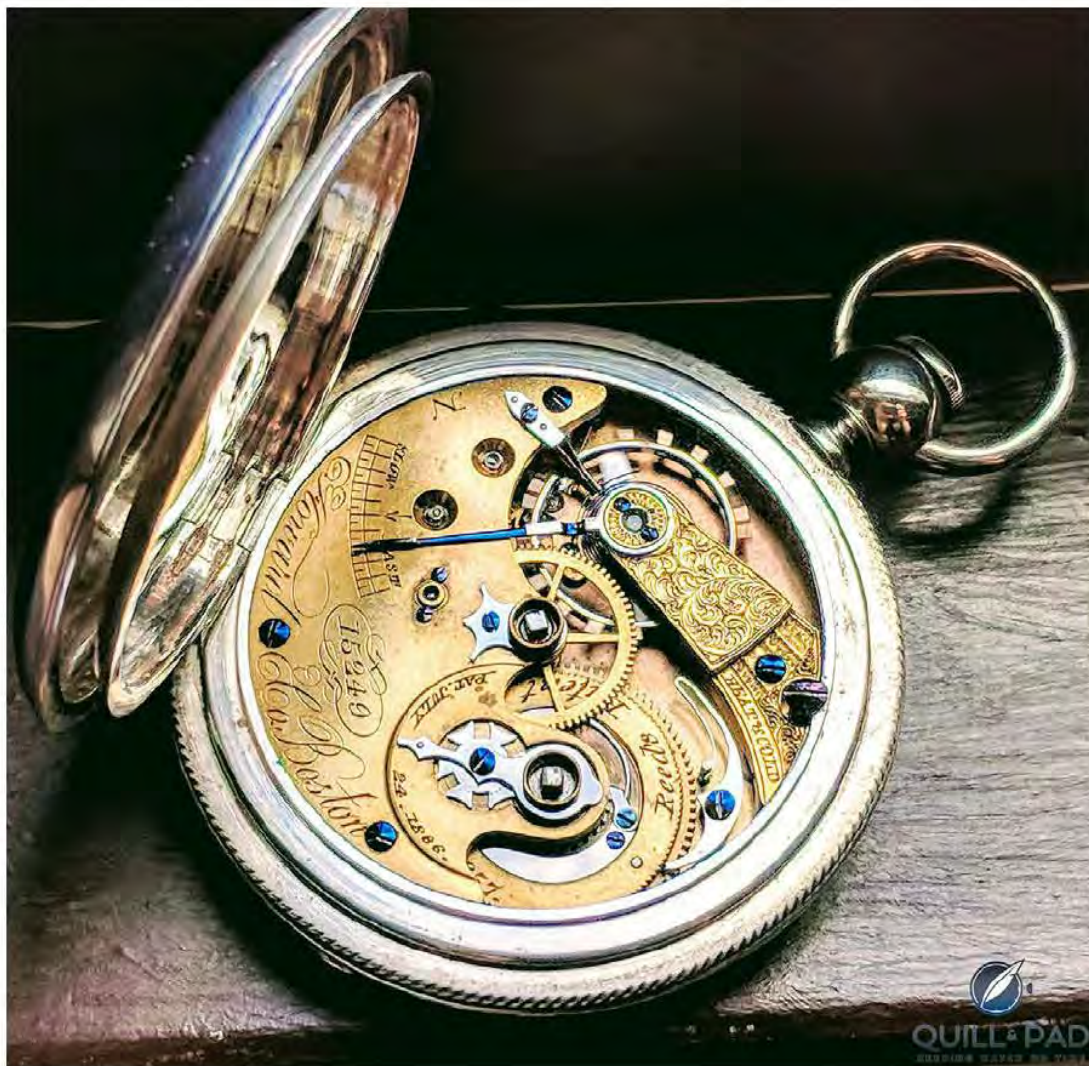
E. Howard and Co pocket watch with square pegs for winding and setting the time with a key (photo courtesy Derek Weinberg)
