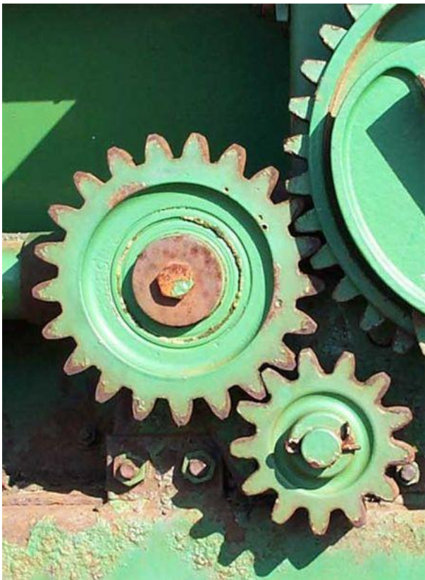
2 gears and an idler gear on a piece of farm equipment, with a ratio of 42/13 = 3.23:1
