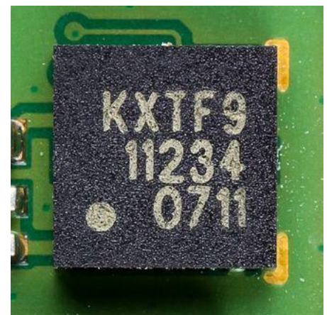
Tri-axis Digital Accelerometer by Kionix, inside Motorola Xoom
