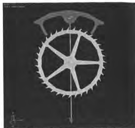
Fig. 1: Model of Graham Escapement in RecurDyn®.
