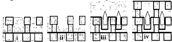
Figure 1: Standard technological sequence used to incorporate air gaps in a specific metal level, hereafter using non-conformal CVD technique. (i) Once the complete realization of a interconnect stack achieved, (ii) a specific lithography step is introduced to define air gap trenches in-between copper lines. (iii) Then a dielectric liner and a dielectric IMD are successfully deposited to create air cavities. (iv) After that, the interconnect stack is completed using a standard dual-damascene architecture (after [9]).
