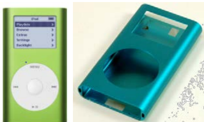
One-Piece Housing—iPod mini (2004)
