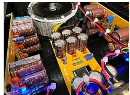
Interior of high-end linear power supply with toroidal mains transformer.
