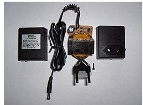
An AC adapter disassembled to reveal a simple, unregulated linear DC supply circuit: a transformer, four diodes in a bridge rectifier arrangement, and an electrolytic capacitor to smooth the waveform
