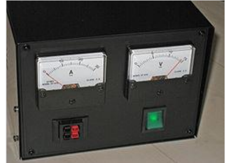
A simple general-purpose desktop power supply used in electronic labs, with power output connector seen at lower-left and power input connector (not shown) located at the rear
