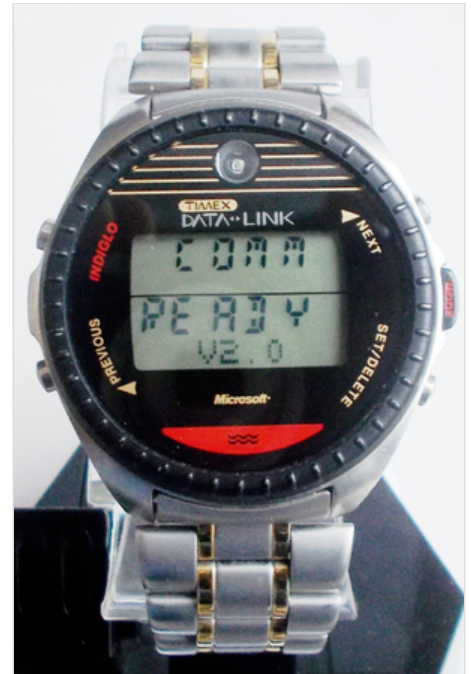
The model 150 with steel bracelet (model 69737) in PC-communication mode. The optical sensor is clearly visible at 12 o' clock on the face of the watch. The Microsoft logo is also visible. The wave pattern below the Microsoft logo indicates that the watch is water resistant. The leather strap version of the watch (model 69721) was worn by commander William Shepherd during Expedition 1 and cosmonaut Mikhail Tyurin, Expedition 14, on the ISS .
