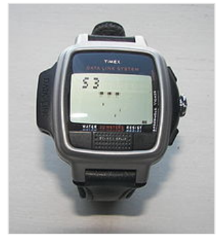
Datalink USB Dress edition with Invasion video game wrist app. (Three lives remaining). The watch crown ( i-control ) can be used to move the defender left to right and the fire control is the Start/Split button on the lower side of face of the watch at 6 o' clock. The pixels of the invaders appear slightly blurred upon picture magnification because of the animation of the aliens. The faint pixels diagonally to the left of the defender block are pixel traces of alien missiles.
