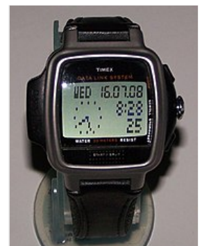
Datalink USB dress edition with a WristApp installed to display time in analog digital format
