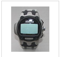
Datalink Ironman USB in screen saver mode. The screen saver activates automatically when the display is at :00 seconds.
