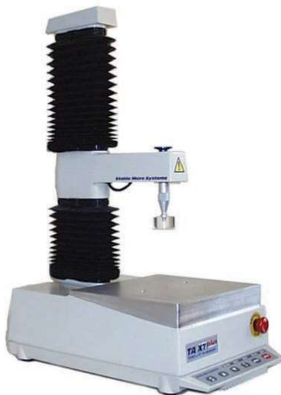
Figure 6. Image of a Texture Analyzer (TA.XT Plus, Texture Technologies, Scarsdale, NY).
